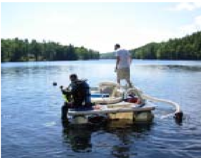
At left, divers and the surface tender prepare to start harvesting with the D.A.S.H. unit. At right, the surface tender clears the catchment net and transfers milfoil plants to a container for measurement and subsequent disposal.
